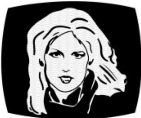
Fig. 11-5. A herringbone pattern caused by adjacent channel interference.
