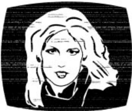
Fig. 11-8. Bright static caused by electromagnetic interference.
