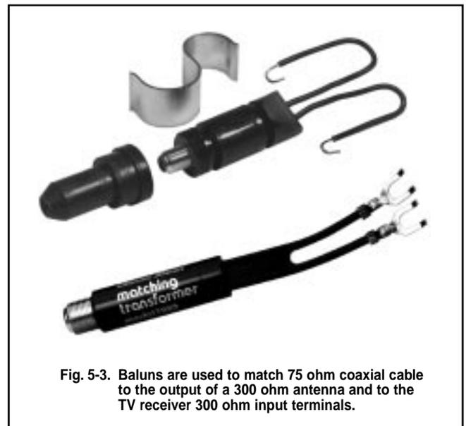
Fig. 5-3. Baluns are used to match 75 ohm coaxial cable to the output of a 300 ohm antenna and to the TV receiver 300 ohm input terminals.
