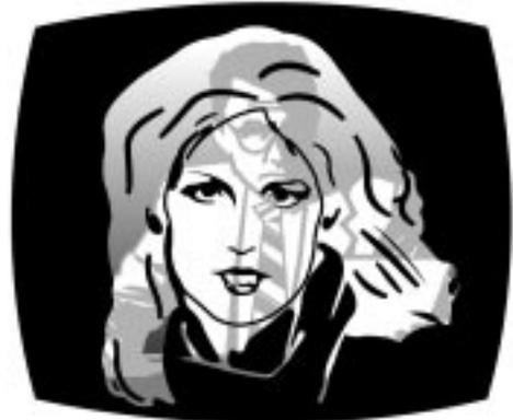
Fig. 11-6. Co-channel interference.
