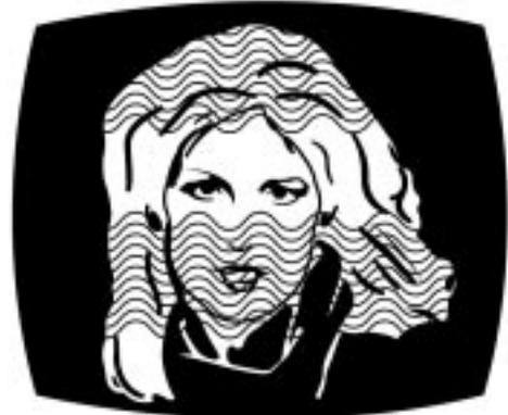
Fig. 11-9. A herringbone pattern caused by FM interference.
