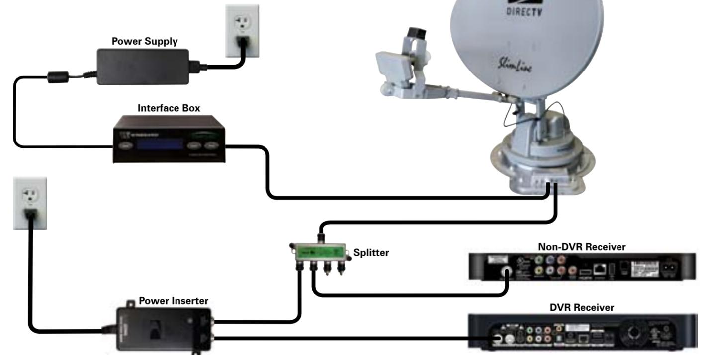
FIGURE 9. Setup Option 2 with fully assembled antenna
