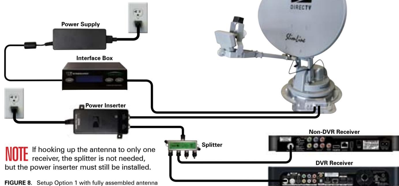
**NOTE** If hooking up the antenna to only one receiver, the splitter is not needed, but the power inserter must still be installed.
