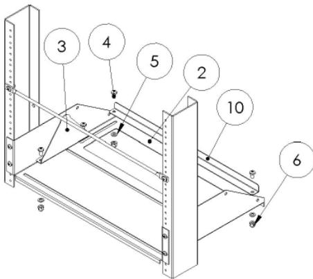
Step 4: Attaching the triangle plates
