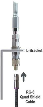
**Antenna Mounting** - The antenna L-bracket (**Figure 1**) should be first mounted in place to either a wall (**Figure 2**), chimney or a pole (not larger than 2 inches in diameter) as shown in **Figure 3**. The antenna should be as high above ground level as practical and as far away as possible from local AM interference sources and any structure (including aluminum siding) that could block reception.
